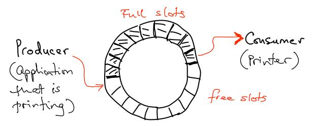
Obviously, the requests should be queued in an FCFS buffer of a finite size *B*, in the spooler. You need to implement the buffer as a circular array as shown in the figure, for better use of memory. In this *bounded-buffer* or *producer-consumer* problem, you can think of the clients as request producers and the printers as consumers.
