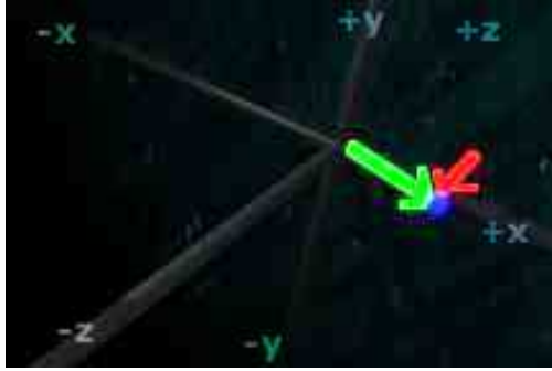
Figure 4: Instead of a distance along the z axis, the vector's (green) z component (red) can be thought of as the distance from the point (blue) to the plane encompassing the x and y axes.
